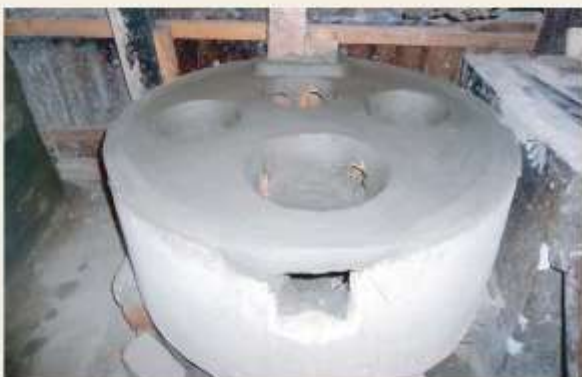
Four Burner Improved Cook Stove for Tea Stalls (Model)
